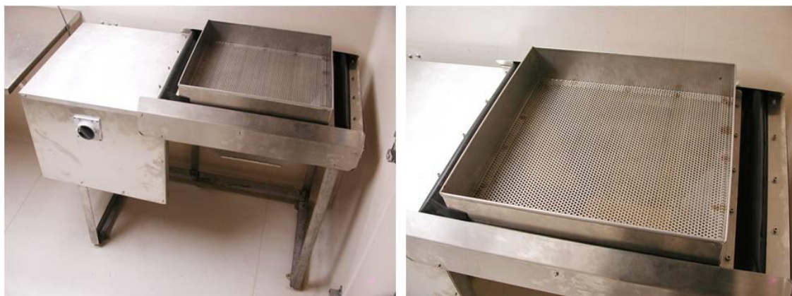
Figure 9. Mechanical sieves constructed for use in the quarantine cubicles. The apertures of the sieve inserts were different sizes for the 2 species.
